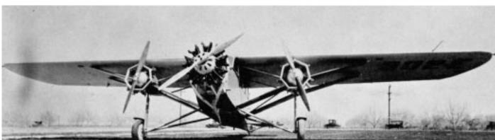
The Bach Air Yacht, built in Van Nuys, California. This one has a Hornet in the nose, two Comets outboard.
