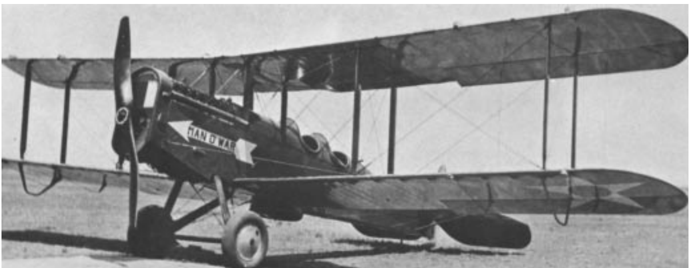
Military planes of 1925 included the de Havilland DH4. Note spare tire carried on belly.
