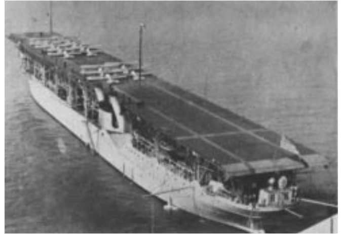
The Navy's first carrier, USS Langley CV1 , commissioned in 1922. Vought biplanes are parked on deck, which was 64 feet wide, 534 feet long. (Leon Cuddeback)
