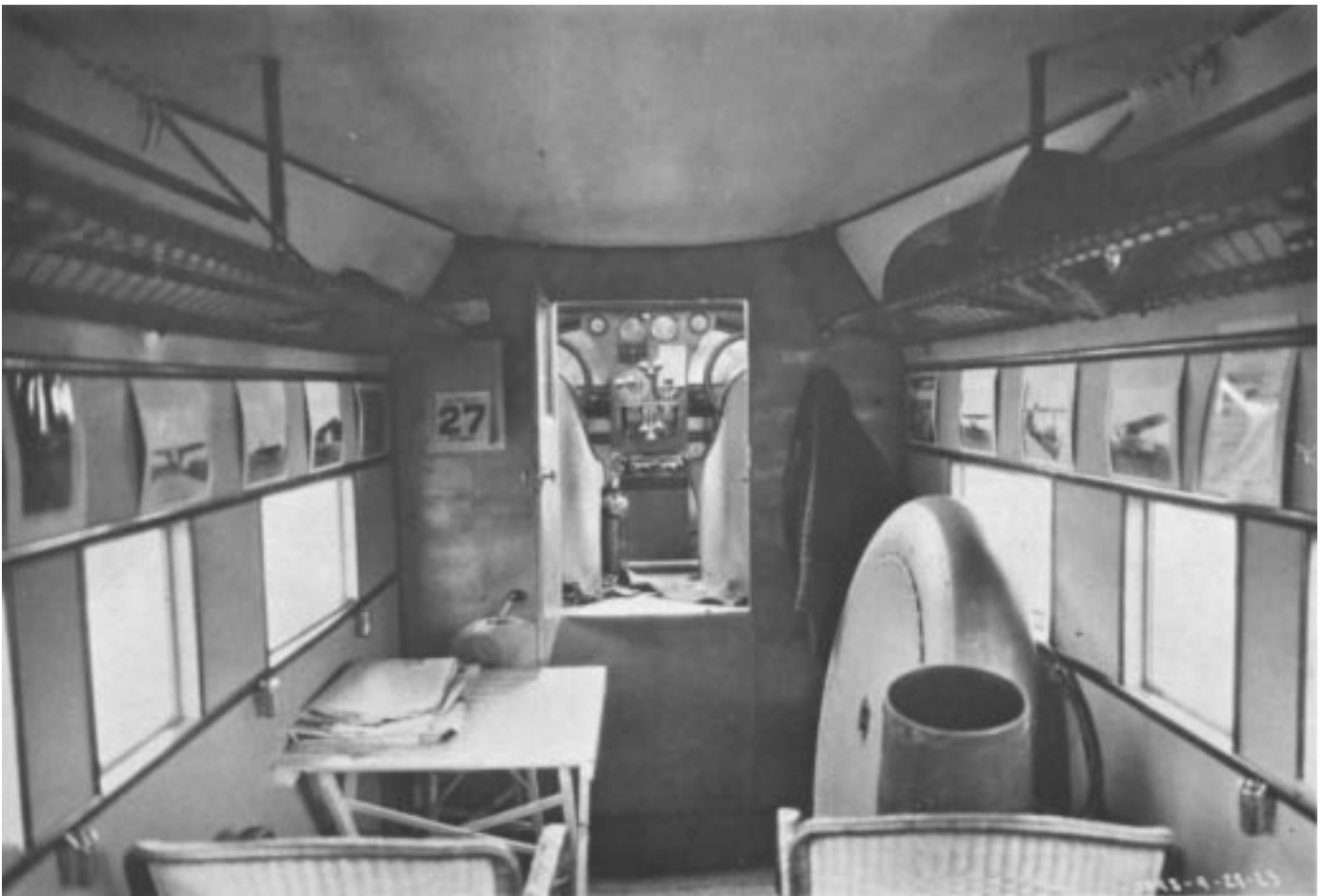
Interior of Fokker. Spare wheel at right, calendar and desk at left, advertising placards line walls below hatracks. Crank at left front may be cabin heat control. Ford Airport Rules note is propped up on simple instrument panel.
