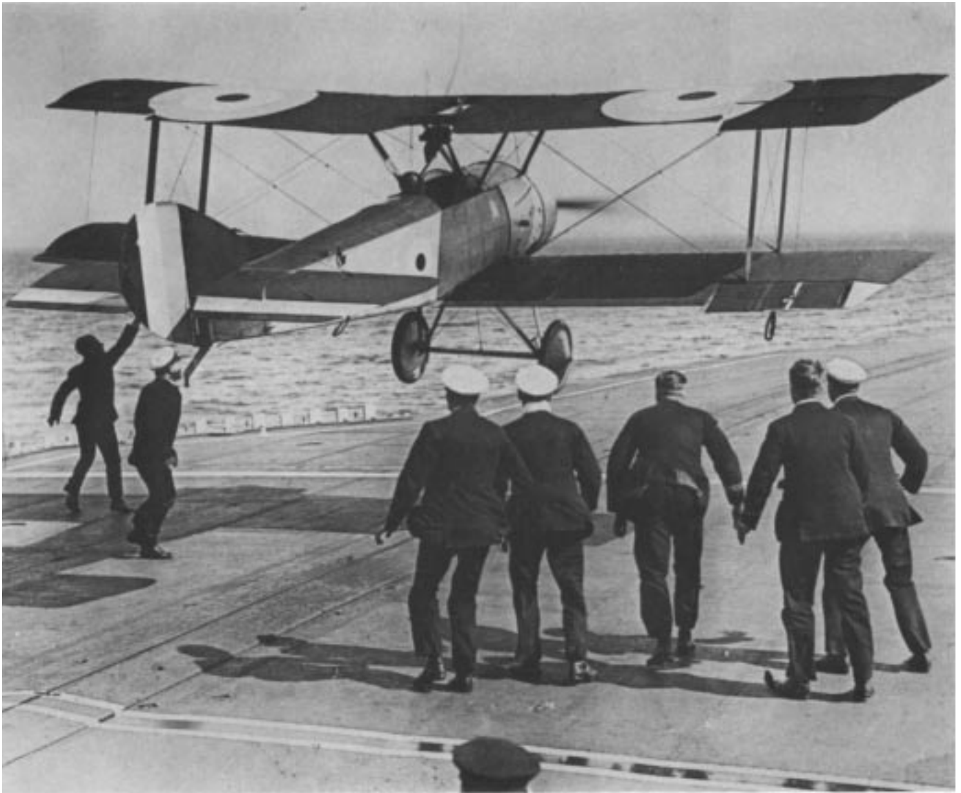
A carrier exercise in the British Navy in 1917, only eight years before the first air tour ventured forth. Sopwith Pup lands and is dragged to a stop by ground crew on makeshift platform built across forward deck of HMS Furious . (Imperial War Museum)
