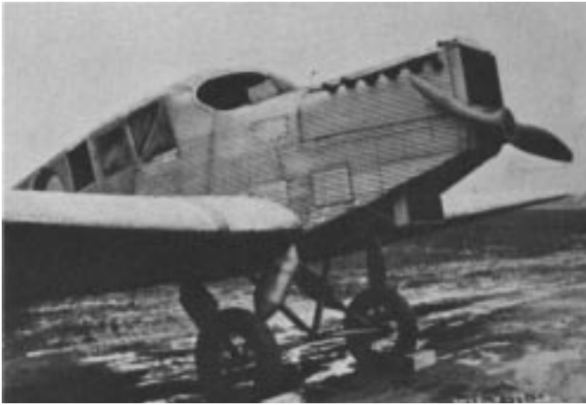
The Junkers F-13L. Thick cantilever wing was first patented by Hugo Junkers in 1910, used on a German fighter plane in 1915, and on the first 4-place F13 in 1919.
